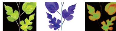
Figure 5. Illustration of an optically addressed image with negative photo mask. (Left) Regular photograph of the original digital image. (Middle) Negative photo mask made of PET. (Right) Image optically written on the display cell.
